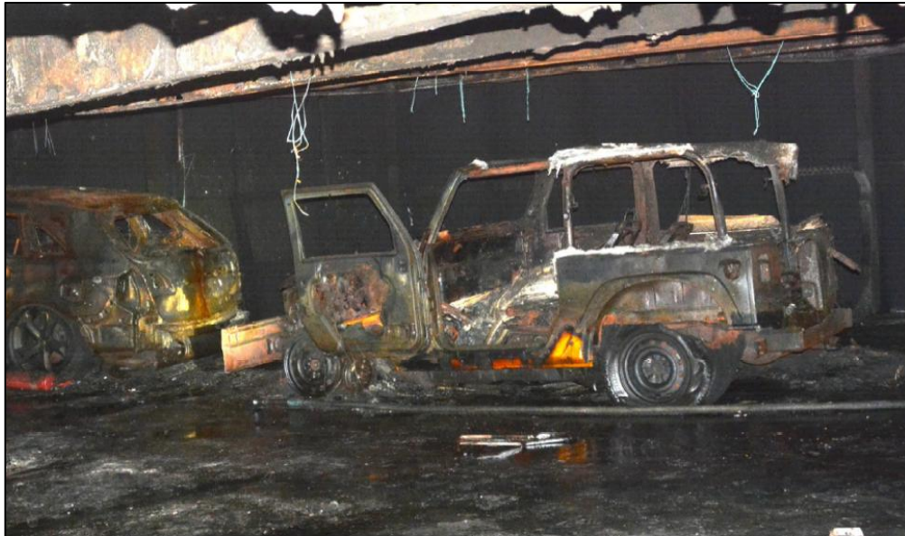
Photo 11. The pusher vehicle experienced a transmission failure, serving as the origin and cause of the fire on deck 10.
