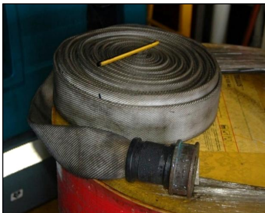
Photos 7 and 8. Vessel's 1½ inch fire hose and coupling.
