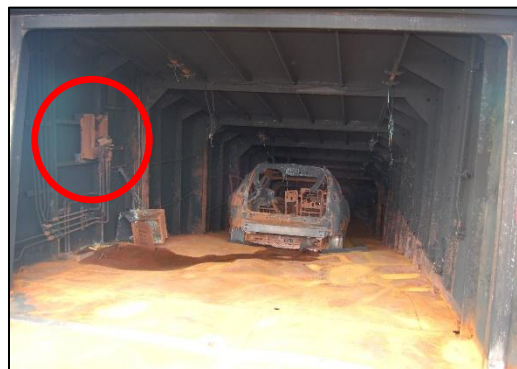
Photo 6. Inside the WTD, showing the door controls on the left.
